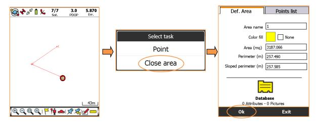
The operation creates a boundary joining the point 3 and 1 with a line. The area feature has been created.
