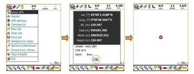
Once connected, GeoGis shows the GPS coordinates table with the geographic and cartographic coordinates of the current GPS position and information about Datum and map projection. Tap **OK** to go back to the map display.
