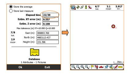
If Step 3 and 4 requires longer time than the memorization of the GPS point (elapsed time>storage time), the measurement cycle is extended till the Database completion.
