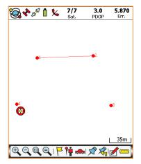
Repeat Step 3 to link the remaining points and to create a closed boundary.
