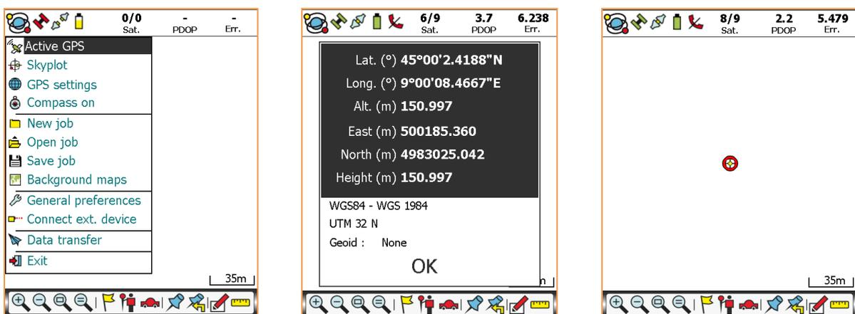
Once connected, GeoGis shows the GPS coordinates table with the geographic and cartographic coordinates of the current GPS position and information about Datum and map projection. Tap OK to go back to the map display.
