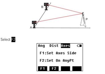
Step 1: Measure the distance to Point A and B, then press F4 to next step.
