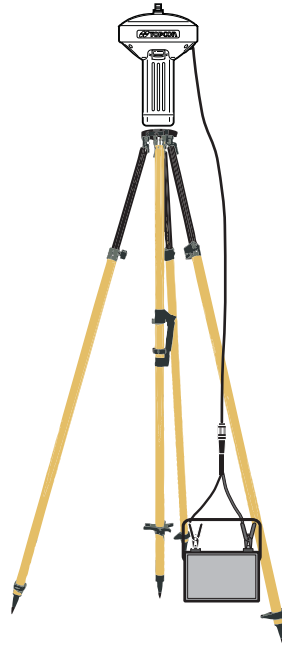
Figure 16: Connect an Auxiliary Battery and the Receiver
