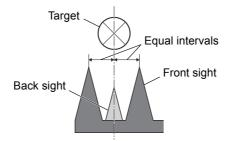
**Vertical direction**: a position where you can see the tops of the front sight and back sight at the same height of the target's center.
