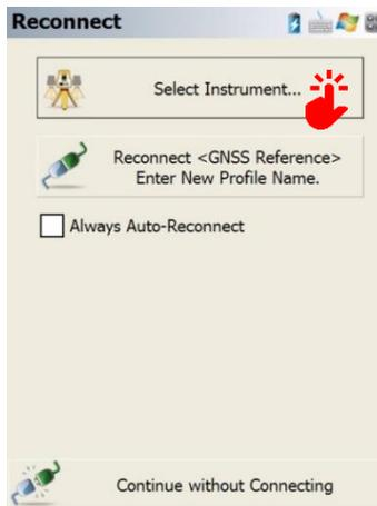
Choose *GNSS Reference* as the *Instrument Type*, which means this receiver will be defined as Base.
