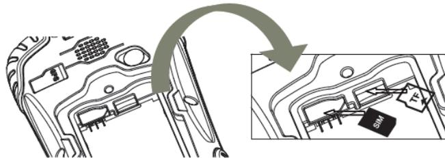
Installing the battery, turn the lock clockwise to the end (SIM card: The missing angle corner of SIM card will be at the lower right corner).
