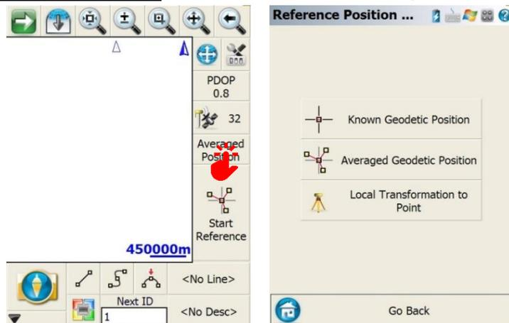
Click **Start Reference** after that. Enter to *Average Position* screen. Click **Modify Antenna Height** to input the height of antenna.
