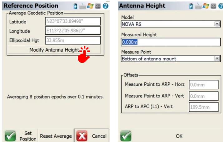
Click **Set Position** to finish the setting of reference position, and select whether to save the reference point to the point database according to your need. Then you will enter to the interface of *Link Configure*.
