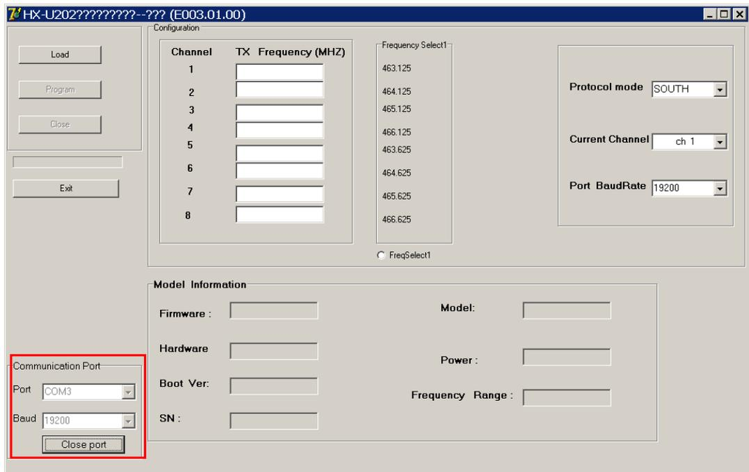
d. Power on the radio and click load ASAP, and then the software will get the radio parameters
