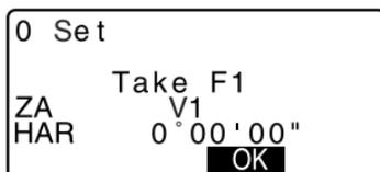
4. Accurately sight a clear target with a distance of about 30m in the horizontal direction with the telescope in Face 1. Press **[OK]**. The vertical angle V2 is displayed under "Take F2."
