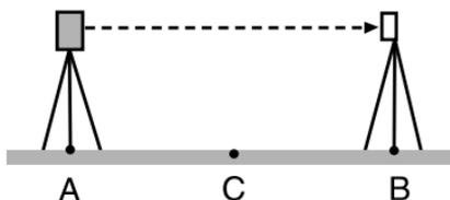
2. Precisely measure the horizontal distance between point A and point B 10 times and calculate the average value.
