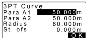
8. Press **[OK]** in the screen shown in step 7 to calculate the coordinates and follow-up distance of the KA1 point, KE1 point, KE2 point, KA2 point. The results are then displayed on the screens shown here. Press **[F5]**/**[F6]** to switch between <3PT Curve/KA1>/<3PT Curve/KE1>/<3PT Curve/KE2>/<3PT Curve/KA2>.
