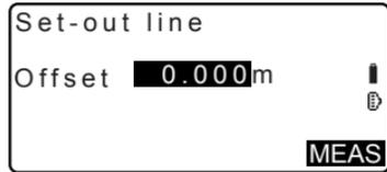
3. Sight the target and press **[MEAS]** on the screen of step 2.
