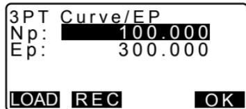
6. The IA ang (intersection angle), direction (of curve), BP-IP (BP-IP length), and IP-EP (IP-EP length) are calculated from the coordinates of the three input points. The results are then displayed on the screen.
