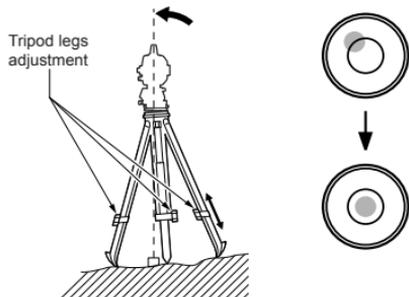
Turn the levelling foot screws while checking the circular level until the bubble is centered in the center circle.
