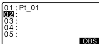
7. Repeat steps 4 to 6 until all points have been measured. Points on an enclosed area are observed in a clockwise or counterclockwise direction.
