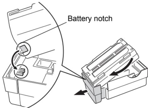
2. Slot the top end of the battery into the battery adapter. The extendable portion of the battery adapter will automatically retract and hold the battery in place.
