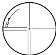
4. Readjust the focus with the focussing ring until there is no parallax between the target image and the reticle.
