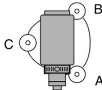
6. Set the tilt angle to  $0^\circ$  using foot screws A and B for the X direction and levelling screw C for the Y direction.
