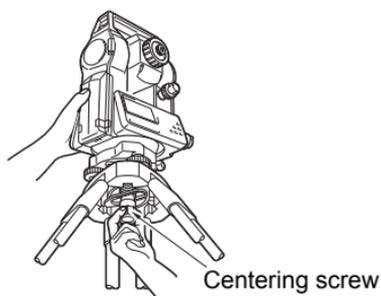
3. Looking through the optical plummet eyepiece, turn the optical plummet eyepiece to focus on the reticle.
