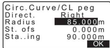
6. Press **[OK]** in the screen shown in step 5 to calculate the center peg coordinates. The coordinates and azimuth angle are then displayed in this screen.
