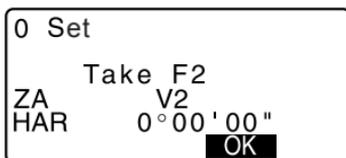
5. Turn the upper part through  $180^\circ$  and clamp it. Then set the telescope in the Face 2 position and accurately sight the same target.
