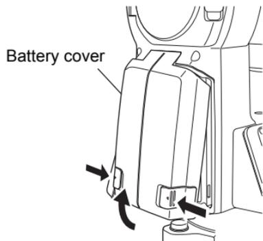
2. Insert the battery with the arrow shown on it downward while pressing toward the instrument.
