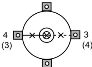
7. Check the adjustment by rotating the upper part of the instrument. The survey point should remain centered in the reticle. If necessary, repeat the adjustment.
