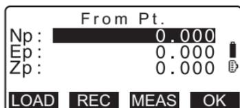
5. Press **[OK]** to use the measurement results of the From point.
