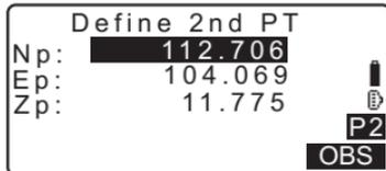
7. Press **[OBS]** on the screen of step 6 to move to observation of the first point.
