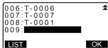
7. Enter the point name of the backsight station for the end point and press **{ENT}**.
