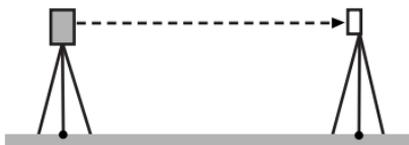
4. While the telescope is in Face 1, sight the center of the target correctly and press **[OK]**.
