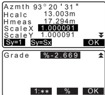
12. Press **[OK]** on the screen of step 11 to define the baseline. <Set-out line> is displayed. Move to setting-line measurement.
