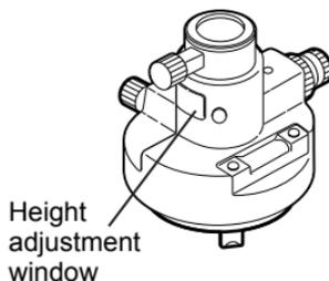
1. Install the tribrach to the instrument height adaptor.
