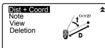
2. Sight the point and press **[MEAS]** to begin the measurement. The measurement results are displayed.
