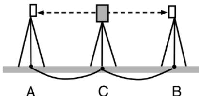
4. Precisely measure the horizontal distances CA and CB 10 times each and calculate the average value for each distance.
