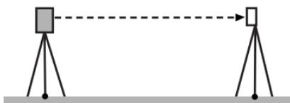
3. While the OBS mode screen is displayed and the telescope is in Face 1, sight the center of the target correctly and read out the horizontal angle A1 and the vertical angle B1.
