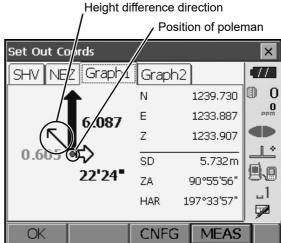
The Graph 2 tab shows the position of the setting out point (square) and the current location of the mirror (circle).
