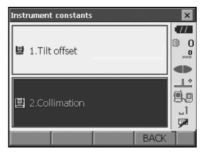
5. While the telescope is in Face 1, sight the center of the target correctly and press **[OK]**. Rotate the instrument 180°.
