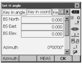
When checking backsight distance, sight the backsight station and press [MEAS]. Press [STOP] to display the distance calculated from coordinates, the measured distance, and the difference between the two. Press [YES] to set the azimuth angle and display <Coord. measurement>.
