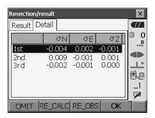
8. If there are problems with the results of a point, align the cursor with that point and press **[OMIT]**. "OMIT" is displayed to the right of the point. Repeat for all results that include problems.
