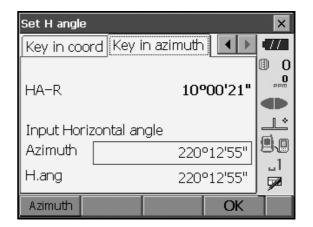
Press [OK] to set the input values. <Coord. measurement> is displayed.
