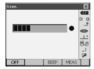
When **[S-LEV]** is pressed, a gauge indicating light intensity is displayed.
