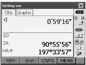
5. Sight the target and press [MEAS]. Measurement begins and the measurement results are displayed.
