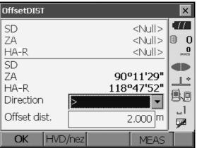
6. Sight the offset point and press **[MEAS]** in the screen of step 5 to start measurement.
