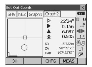
ove the target to find the correct distance (0 is displayed) to the setting out point.
