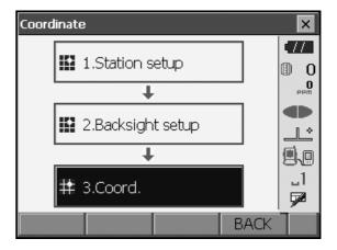
Press **[MEAS]** to start measurement. Press **[STOP]** to stop the measurement. The coordinates of the target point are displayed. Select the "Graphic" tab to display coordinates on a graph.
