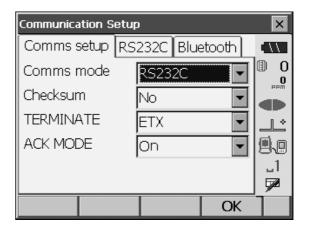
3. Set options in the "RS232C" tab according to the selection made in the "Comms setup" tab.
