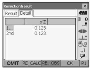
7. If there are problems with the results of a point, align the cursor with that point and press **[OMIT]**. "OMIT" is displayed to the right of the point. Repeat for all results that include problems.
