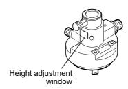
2. Level the instrument and check the position of the bubble of the plate level.
