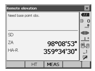
The measured distance data, vertical angle and horizontal angle are displayed.
