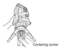
Looking through the optical plummet eyepiece, turn the optical plummet eyepiece to focus on the reticle.
