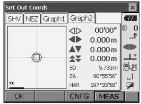
Press [OK] to return to <Key in coord>. Set the next setting out point to continue setting out measurement.
