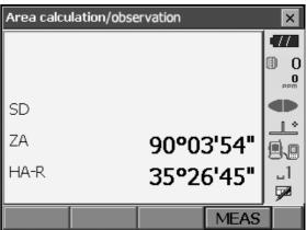
3. The measurement results are displayed. Press **[YES]** to confirm. The value of point 1 is set in "Pt 01".
