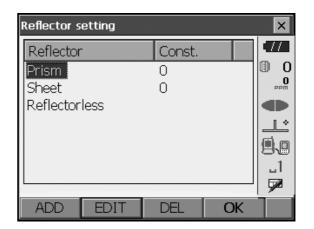
2. To edit a target, select the desired target and press **[EDIT]**. <Reflector/edit> is displayed. Select/input relevant information for the target.
