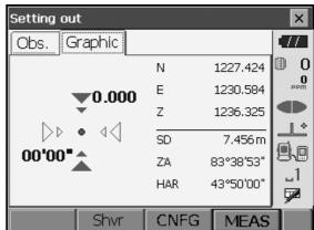
Press {ESC} to return to <Setting out>. Set the next setting out point to continue setting out measurement.
