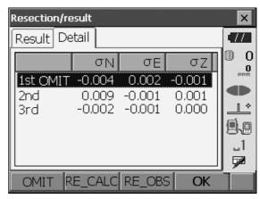
Press [RE\_CALC] to perform calculation again without the point designated in step 8. The result is displayed.
