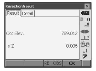
Standard deviation values for each point are displayed in the "Detail" tab.
