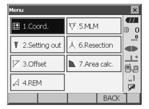
3. Select "Occupy setup" and enter instrument station coordinates,instrument height (HI) and target height (HR).
