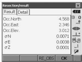
Standard deviation for the northing, easting and elevation coordinates of each point are displayed in the "Detail" tab.
