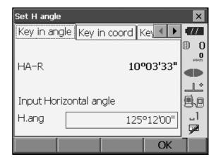
3. Press **[OK]** to set the input values. <Coord. measurement> is displayed.
