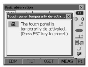
The touch panel cannot be operated while the above message is displayed. Press **{ESC}** to cancel the message and re-activate the touch panel.
