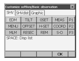
Select the softkey whose allocation you want to change. Tapping a softkey, or pressing {SPACE} when the cursor is aligned with a softkey, will display <Softkey list>.
