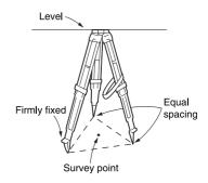
Place the instrument on the tripod head.Supporting it with one hand, tighten the centering screw on the bottom of the unit to make sure it is secured to the tripod.
