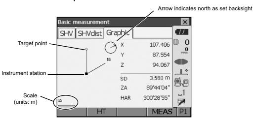
The "Graphic" tab display can be modified using the softkeys in the second page.
