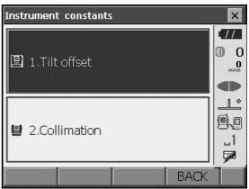
4. Level the instrument until the X/Y tilt angles are ±1'. Wait a few seconds for the display to stabilize, then read the current tilt angle in the X (sighting) direction and Y (horizontal axis) direction.
