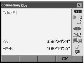
6. While the telescope is in Face 2, sight the center of the target correctly and press **[OK]**.
