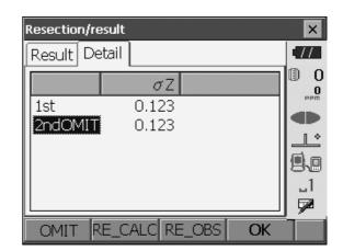
8. Press [RE CALC] to perform calculation again without the point designated in step 7 The result is displayed.
