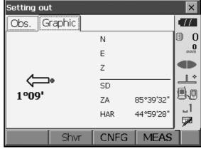
6. Position the target on the line of sight and press [MEAS] to begin distance measurement.
