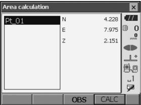
4. Repeat steps 2 to 3 until all points have been measured. Points on an enclosed area are observed in a clockwise or counterclockwise direction. For example, the area specified by entering point numbers 1, 2, 3, 4, 5 or 5, 4, 3, 2, 1 implies the same shape.
