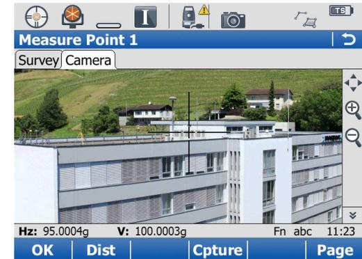
Fine style crosshairs for accurate aiming of the telescope
